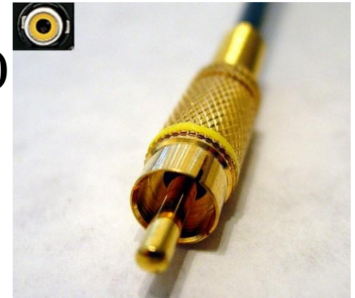
Composite Video Cable and Connection
