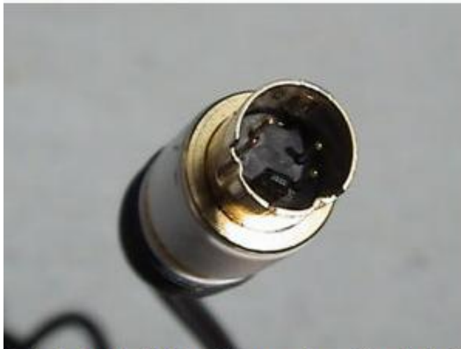
A standard 4-pin S-Video cable connector, with each signal pin paired with its own ground pin.
