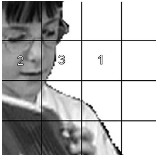
Figure 5.29 VO showing external (1), internal (2) and boundary (3) macroblocks
