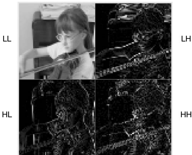
Figure 3.33 Image after one level of decomposition
