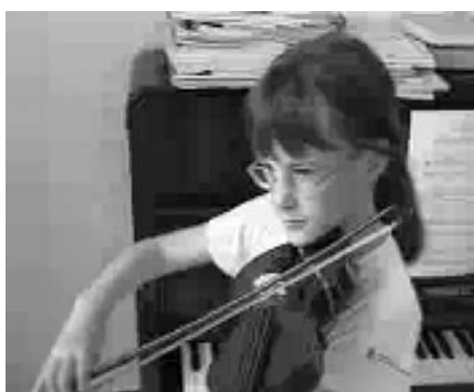
Figure 6.35 Reconstructed, QP = 32 (no filter)
